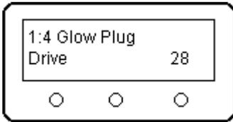
If you have ignition problems (no light off), try increasing the drive a unit or two until reliable ignition is realized.
