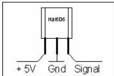
*This hall sensor is available from 5 Bears, encased in a 0.25" / 6.35mm aluminum tube, complete with cable and plug for a direct connection to the ECU. It comes also with 2 rare earth magnets for your installation into the compressor spinner nut of your turbine. Please see [www.5bears.com](http://www.5bears.com) for more details*
