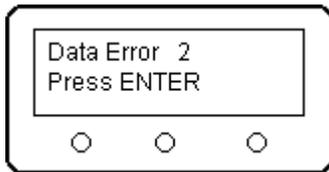
**What you will see:** After power up, or when you have exited a programming session, the ECU has detected a data error. The screen here is displayed, informing you of the error, and prompting you to press the ENTER button. After looking up the error here in the manual, press the enter button, and the ECU will enter the programming mode, allowing you to correct the error.
