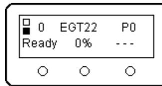
Leave the throttle in idle. Prime, if necessary, by pressing and holding the UP and DOWN buttons simultaneously. Release the buttons. Apply the air to the inlet of the turbine. The rotor should begin to spool up.
