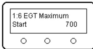
**Page 6: EGT Maximum for Starting:** The 5 Bears ECU allows two maximum EGT values, one for starting, the other for normal run operations. Press Enter, and use the Increase and Decrease buttons to change this value. The Max Start EGT increments by plus or minus 5 degrees Celsius. Press Enter once more to store the new value.
