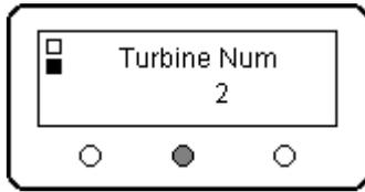
Pressing the Up button, shown here, changes the displayed Turbine Number from 1 to 2. Pressing and holding either the Up or Down buttons will rapidly scroll the value to the lower right. When you are happy with the data...
