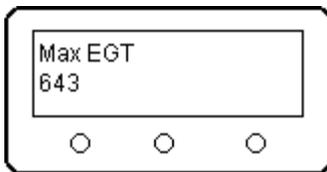
...and then the first data log page becomes visible. Pressing Enter repeatedly will page through the data. No modifications are permitted; the Up and Down buttons are inactive. The first page shows the Maximum EGT encountered during both startup and running of the turbine.
