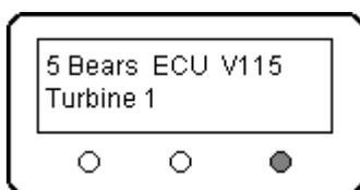
First, connect a battery and turn the power switch ON. While this screen is displayed, press and hold the Enter button, shown here as a dark button.
