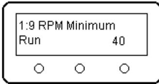
**Page 9: RPM Minimum Run:** This is your turbine's **idle** RPM. Enter the desired target in thousands. During start (and Run, when idle is commanded), the ECU will continually trim the pump output in an attempt to track this RPM. Please see my observations on Idle RPM earlier in this chapter. To summarize, a higher idle is preferable if your model can handle the thrust that such an idle will generate.
