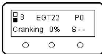
The electric starter has spun the turbine up to 8,000 RPM. Note the S—annunciation, telling you that the starter motor is energized, but neither
