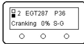
The propane is ignited! Note the EGT rise. Upon detection of successful ignition of the propane, the **I**gnition source is cutoff. **G**as remains on.
