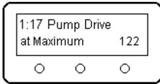
**Page 17: Pump Drive at Max:** During the first live running of the turbine/ECU combination, the turbine will undergo what is called a **Max Run**, a slow acceleration to the programmed Max RPM, to determine a valid pump output value at the “top end”. This value is automatically stored here for viewing by you. Subsequent flights will skip the Max Run as long as the ECU finds this value upon power up. It is dynamically modified during running of the turbine, and the value will change
