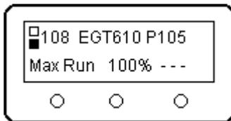
The ECU will command a gentle acceleration. As the turbine accelerates, it will sense your programmed Max RPM and halt acceleration at that point. During the Max Run, if you wish to halt acceleration, simply move the throttle to midrange. The turbine will stabilize at an intermediate RPM. If you wish to continue the Max Run, return the throttle to 100%. If, at any time you wish to idle the turbine, simply retard the throttle to idle, or 0%
