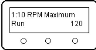
**Page 10: RPM Maximum Run:** Enter the absolute maximum RPM for the turbine. Derating your turbine for both safety and turbine longevity is a good idea. I personally limit my MW-54 (designer max. RPM of 160,000) to 154,000. The ECU does a good job in preventing overspeeds and aggressively reduces fuel flow upon overspeed detection, but a slight derate provides peace of mind and a bit of buffer in case of fuel injector or line failures, or other failures which can cause a sudden surge
