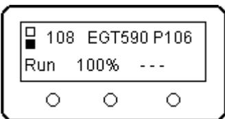
Once Max RPM is reached, the ECU will announce RUN and you will have full, normal control of your turbine. Time for the Max Run will vary, but is roughly 10 to 15 seconds. Full envelope protection is provided, and any faults encountered will be handled by the ECU. Now, retard the throttle and go fly! In the Run mode, any time either 0% or 100% throttle is commanded, the ECU trims the turbine to maintain the appropriate RPM.
