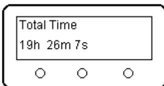
The final log page is the elapsed, total time for the turbine. This cumulative includes *all* of the turbine sets. If you wish to track elapsed times for separate turbine sets, it must be done manually.
