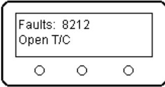
Finally, after all the logged data has been displayed, pressing Enter will reveal any faults encountered during the run. If there is any question as to the faults revealed, make a note of the number to the right of the Faults: annunciation, for reporting to me at 5 Bears Engineering. Here, the ECU has reported an Open T/C, or open thermocouple error. See the Errors section for more detail. Pressing Enter one last time will return you to the normal ShutDown display. The ECU must be reinitialized
