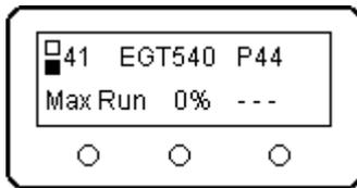
The Max Run is the only “hot” programming done for the ECU. Its purpose is to create a fuel pump mapping, telling the ECU what approximate pump drive level is required to allow the turbine to approach its programmed maximum RPM. This *must* be done at least once, and the model should *not* be flown until it is complete. Secure the model, stay clear of exhaust and rotational planes, and apply full throttle. *There will be no acceleration of the turbine until the throttle reaches 100%.*
