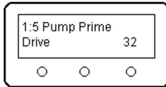
**Page 5: Pump Prime Drive:** Set up your turbine with a fuel supply and pump either in the model or in a position similar to the model on a test stand. Important considerations are the height of the fuel tank, pump, and turbine relative to each other. Press enter. The Pump Prime Drive reinitializes to 0. Pressing Increase will begin powering the pump.
