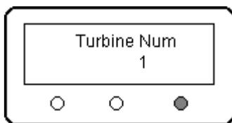
...followed by the opening page of the Setup mode. Each programmable data item is displayed as a separate page. Here, the page is telling us that the ECU is ready to program Turbine 1. The ECU can store complete data sets for 3 different turbines. Each turbine data set must be separately programmed. To change the Turbine Number, press the highlighted Enter button again.
