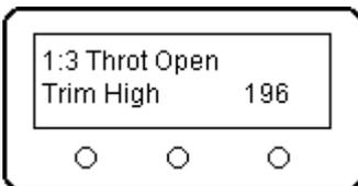
**Page 3: Throttle Open, Trim High:** Throttle fully open (forward) and throttle trim fully high. During flight, the throttle trim tab controls the turbine operation. If the trim is ever below mid-range and the throttle reduced to idle, the ECU will receive a shutdown signal, and initiate the shutdown procedure. Keeping the throttle trim high will allow the turbine to operate normally, from idle through max power.
