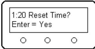
**Page 20: RESET TIME?** The ECU will log all cumulative elapsed run time from start initiation to shutdown. This value will be displayed during the log view session. If you want to reset the elapsed time to zero, press and hold the enter button for 5 seconds. The time will be reset, and the ECU will reenter its normal program mode.
