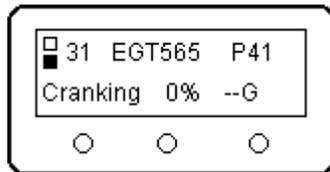
As soon as the propane ignition is confirmed, the ECU begins a controlled introduction of the liquid fuel, and tracks EGT and RPM right up to idle. If electrically starting, the starter circuitry will cutoff when the RPM reaches the preprogrammed Starter Cutoff RPM. If air starting, remove the air at approximately Idle RPM minus 3 or 4 thousand. Overshoots (sometimes large) of idle RPM during air starts are common and no cause for concern. The turbine is now started!
