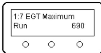
**Page 7: EGT Maximum for Run:** Press Enter and modify this value as desired, keeping the value at or below the turbine designer's stated maximum EGT. The Max Run increments by plus or minus 5 degrees Celsius. Press Enter once more to store the new value.
