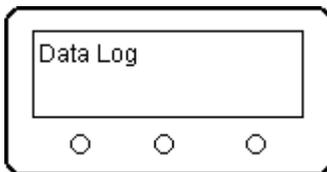
After the cooling cycle is complete, the ECU will display a screen similar to the **Normal Shutdown** LCD display shown above. Press the Enter button to view the data log. This screen is briefly displayed...
