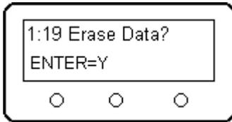
**Page 19: Erase Data?** To erase all of the data for only the turbine being programmed, *press and hold* the ENTER button. The LCD display will show “Hold to Erase”. If you continue pressing the enter button for approximately 5 seconds, the data for the specific turbine set will be erased, and all values reset to 0. Releasing the button early will abort the erase procedure, and the data will be retained. If you erase data for Turbine 2, Turbines 1 and 3 will still retain their data.
