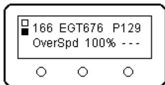
**What you will see:** If you have the LCD attached and are bench running, the lower line RUN mode is replaced with the fault detected. If there is more than one fault active, the most serious fault is displayed. Here, the ECU has detected a rather severe overspeed of 166,000 RPM. If the LCD display shows a fault, it is an indication that the ECU is, in fact, handling the fault.
