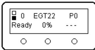
Open the throttle (stick fully forward) and hold there for a few seconds. The turbine primes itself by briefly advancing the fuel, avoiding air bubbles and pump cavitation. Retard the throttle to idle when priming is completed. Start is now initiated.
