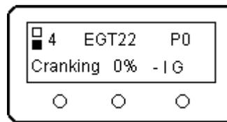
When the ECU senses 3,000 RPM or greater, it will turn on the ignition and the gas, and await propane lightoff. You should remove air when
