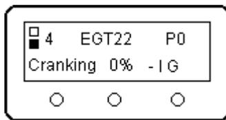
The starter motor has deenergized, and the turbine is decelerating. Ignition and Gas are both switched on in an attempt to obtain propane ignition.
