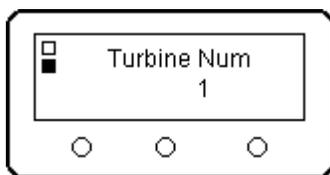
The Enter button does two things with the ECU. First, it tells the ECU that you want to change the current data. After pressing Enter above, an animated widget appears, which consists of a small box that rapidly bounces up and down. This indicates that the displayed data may now be altered using the Increase (middle) and Decrease (left) buttons.
