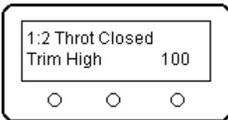
**Page 2: Throttle Closed, Trim High:** Again, press the Enter button to tell the ECU you wish to enter a new value. Be sure the R/C equipment is still properly attached and powered on. Close the throttle (stick fully aft), and run the throttle trim fully high. Press Enter once more to store the new value.
