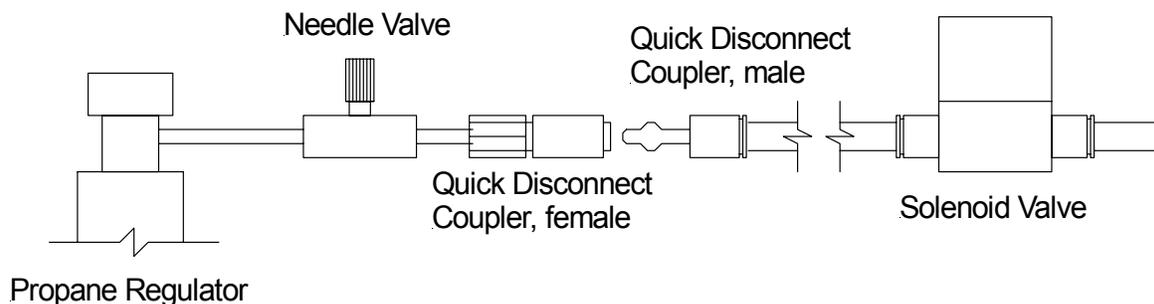
Starting on the left, we have a propane bottle with a regulator. This is fed into an inline needle valve, which in turn is fed into a female Quick Disconnect coupler. This assembly is part of your flight line equipment and is external to the jet.
