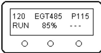
The LCD Data Terminal is laid out as shown. There are three tactile buttons below the LCD bezel. The RIGHT button is the ENTER button. The left button DECREASES the value of the data during programming, and the middle button INCREASES the value of the data. See the programming section for more information on button functionality.
