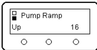
Any time Run is annunciated, three of the programmable values may be altered “live”, while the turbine is running. These are the Pump Ramp Up, Pump Ramp Up Profile, and Pump Ramp Down values. To access these, press the enter button once. Pump Ramp Up is displayed, and the current value shown. Press the up or down buttons to adjust the value; pressing enter again will shift to the Pump Ramp Up Profile page. Adjust this value to your liking. One more press of Enter will display
