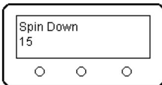
The third page shows the bearing spin-down timing value that the ECU recorded between 18,000 and 2,000 RPM. The actual time is not critical, and will vary widely between turbine types. New bearings should show consistent spin-down times for many runs. If the time suddenly decreases, it may be a sign of bearing wear. It is good practice to record both spin-down time and run time, shown next, in a log book.
