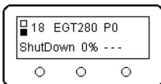
After your jet has landed, taxi back to the pad and shut the turbine down by reducing the throttle to idle and run the throttle trim fully aft. The ECU will hold idle for a few seconds, and it will then shutoff the fuel. Here, the ECU has detected the user Shutdown signal that is now annunciated on the LCD. The pump is off, and the RPM is in the process of decaying through 18,000. EGT from the still hot turbine is 280. Between 18,000 and 2,000 RPM, the time for the spool down (bearing check) is
