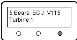
Yes. Turn on the ECU. When you see this screen, press either the Up or Down buttons immediately. You will be shown the logged data and the faults encountered on the previous run. As soon as the next start is initiated, this data will be erased.
