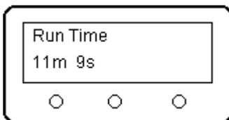
The fourth page of the data log displays the Run time, from initiation of start to shutdown. The display format is in minutes and seconds.
