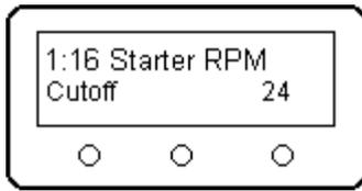
**Page 16: Starter RPM Cutoff** is the value that determines the RPM at which the starter motor is turned off during startup of the turbine. The value must be at least 5,000 RPM less than programmed Idle RPM.
